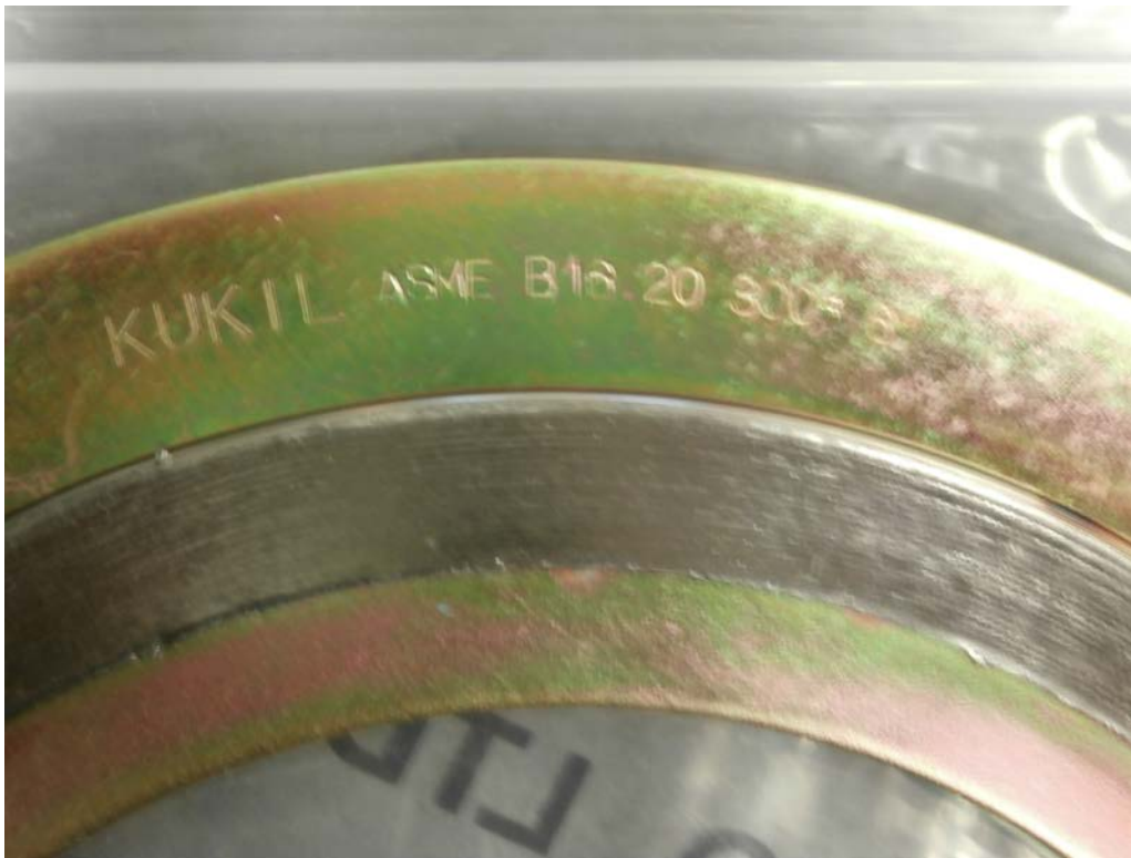
Test Gasket Prior to Burn
