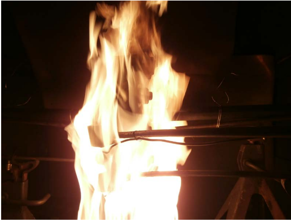
Test Gasket During Burn
